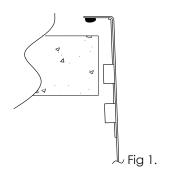
9. Turn the bolt on the inset clips until the serrated cup is nearest to its own "L" shaped hook, Hang the all the inset bolt clips into the top hook of the sink clip hooks, space all the clips supplied evenly around the perimeter. Once done <a href="mailto:very loosely">very loosely</a> tighten the clips so they are close to the underside of the worktop. Now double check the sink is still central to the cut-out hole and is straight to the worktop edge.
