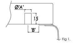
4. Fill the reverse face bracket holes with good quality 2-part epoxy adhesive. Push the metal inserts fully into the holes (this might be easier with the screw inserted), let the adhesive cure before any further assembly. Important: Unscrew the screw from the insert before the adhesive has fully cured to avoid the screw becoming stuck in the insert.
