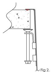
10. Progressively tighten the inset clip bolts in a staggered clockwise order similar to fig. 3 to ensure the sink does not skew or rotate whilst it is fixed.
